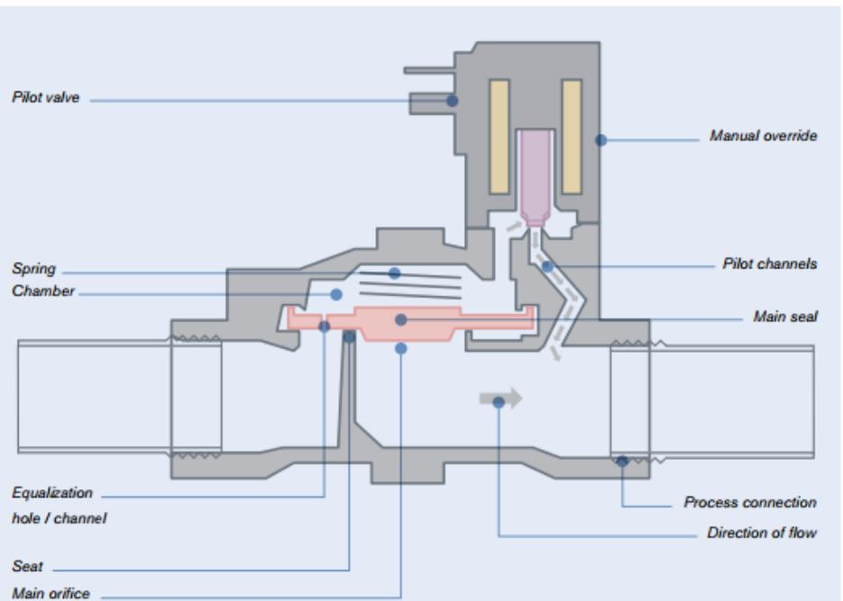
Opening large orifices using the direct acting method would require enormous and expensive coils. Therefore servo assisted valves use the power of the fluid to open the flow channel by controlling a small pilot channel to alter the forces on a larger main seal.
