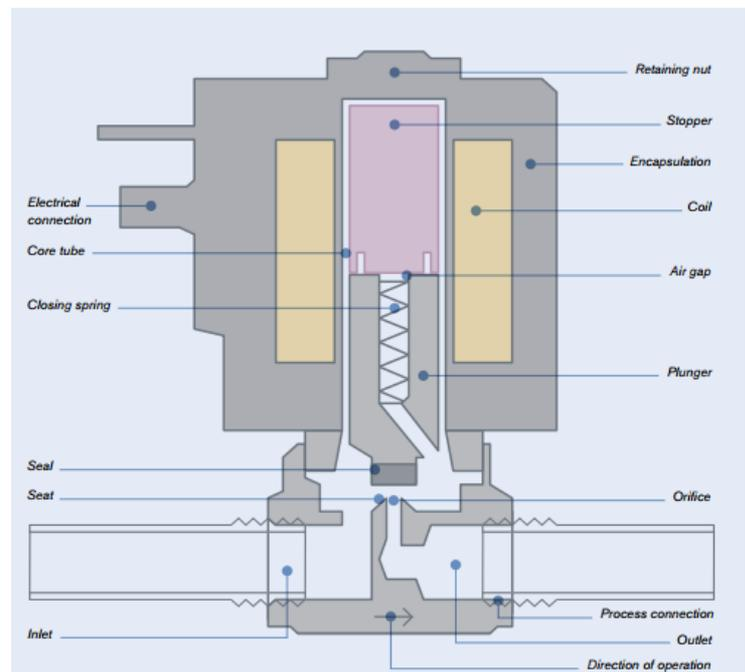
Solenoid valves are the most frequently used control elements in fluidics. Their tasks are to shut off, release, dose, distribute or mix fluids (liquids and gases). They are confronted with many different requirements in a plethora of application environments and must offer:
